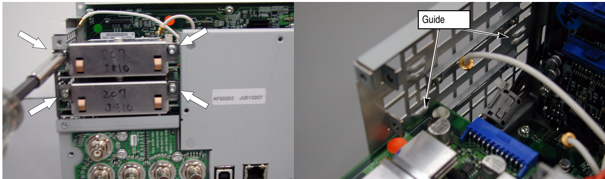
Figure 6-8: Output board removal
