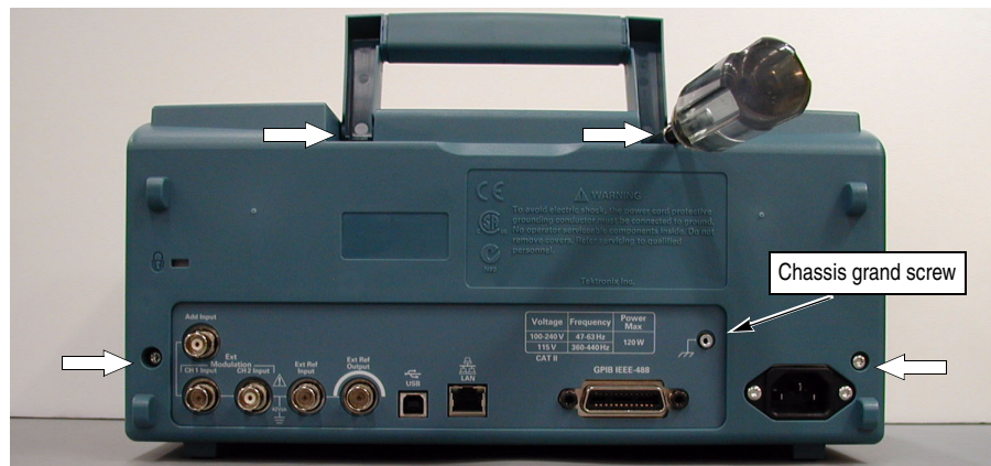
Figure 6-3: Rear case removal
